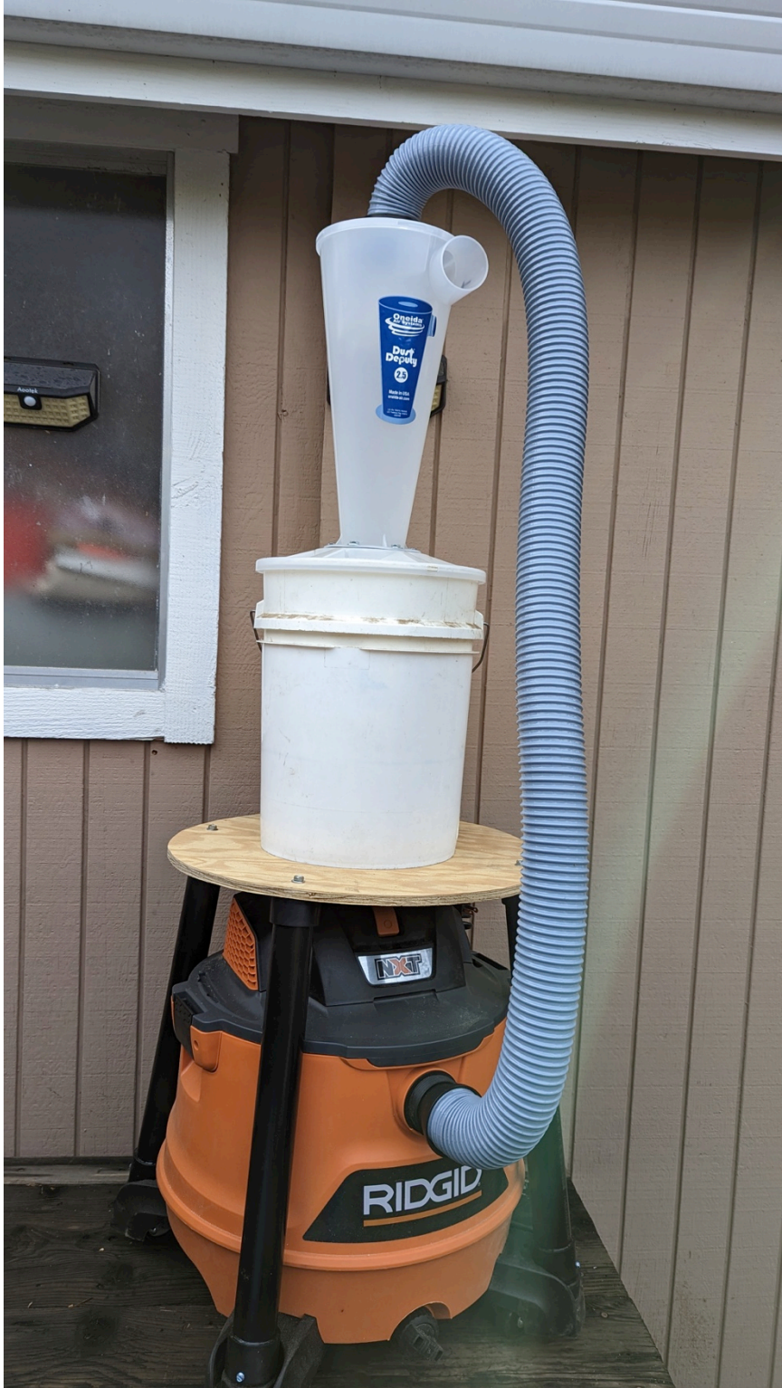
Photo #5 Completed Dust Separator
